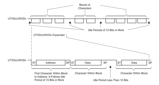
The URXWIE bit is used to control data reception in the idle-line multiprocessor format. When the URXWIE bit is set, all non-address characters are assembled but not transferred into the UxRXBUF, and interrupts are not generated. When an address character is received, the receiver is temporarily activated to transfer the character to UxRXBUF and sets the URXIFGx interrupt flag. Any applicable error flag is also set. The user can then validate the received address.
